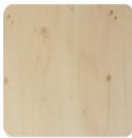
**C:** Supports strong variation of dark color, black knots and some manufacturing defect, taking care that it does not affect the strength of the board.
